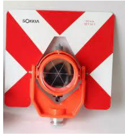
Fig: Reflector used with EDM and Total Station
