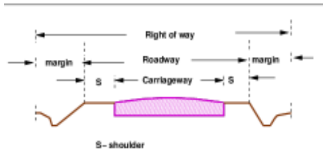
Figure : A typical Right of way (ROW)
