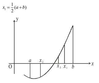
if f(x) = 0, then  $x_1$  is the root of equation f(x) = 0. Otherwise the root lies between a and  $x_1$  or  $x_1$  and b according to  $f(x_1)$  is positive or negative. Then we bisect the interval and continue the process until the root is found to desired accuracy.
