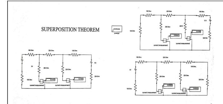
Current through Load Resistor(R<sub>L</sub>) 200 Ohms:
