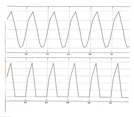
**<u>CONCLUSION:-</u>** From the above experiments we able to draw the single phase half wave uncontrolled rectifier by using simulink.
