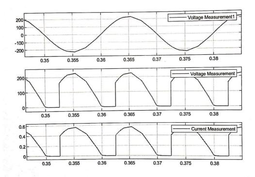
**<u>CONCLUSION:-</u>** From the above experiments we able to draw the single phase full bridge controlled rectifier by using simulink.
