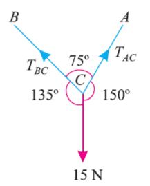
Applying Lami's equation at C,
