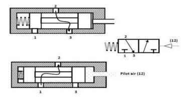
In normal position, the working port (2) is closed to the pressure port (1) and open to the exhaust port (3). When the compressed air is applied through the pilot port (12), the spool is moved against the spring. In the actuated position, the working port (2) is open to the pressure port(1) and closed to the exhaust port(3). Thus, the application of the compressed air to the port 12 causes the pressure port (1) to be connected to the working port (2).
