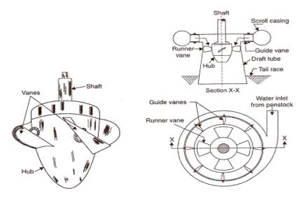
The Kaplan turbine is an inward flow reaction turbine, which means that the working fluid changes pressure as it moves through the turbine and gives up its energy. The desi combines radial and axial features.
