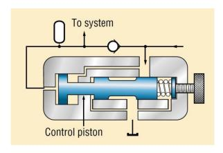
The hydraulic pressure control valve plays a vital role in controlling the leakages and bursting of pipes. Pressure control valves regulate the pressure of the fluid passing through the pipe by releasing the excess pressure. These valves maintain the pressure as entered manually by the operator.
