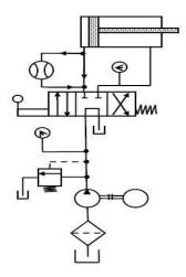
The circuit diagram to control double-acting cylinder is shown in Figure The control of a double- acting hydraulic cylinder is described as follows:
