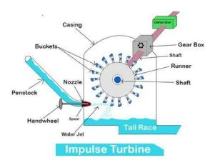
The Pelton wheel or Pelton turbine is tangential flow impulse turbine. The water strikes the bucket along the tangent of the runner. The Energy available at the inlet of the turbine is only Kinetic energy. The pressure at the inlet and outlet of the turbine is atmospheric. The turbine is used against high head.
