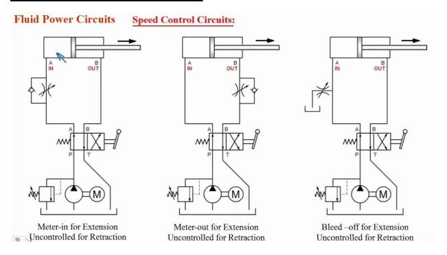
In pneumatic system, cylinder movement may be jerky because air is compressible. As air flow into a cylinder, as pressure increases slowly unit it generates the break way forge needed to start the lord moving .Because the subsequent force needed to keep the load moving as always less than the break way force, the air in the cylinder actually expand.
