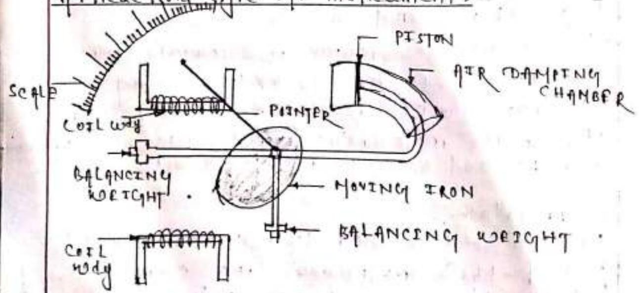
(Fig: Attraction type MI instrument)
