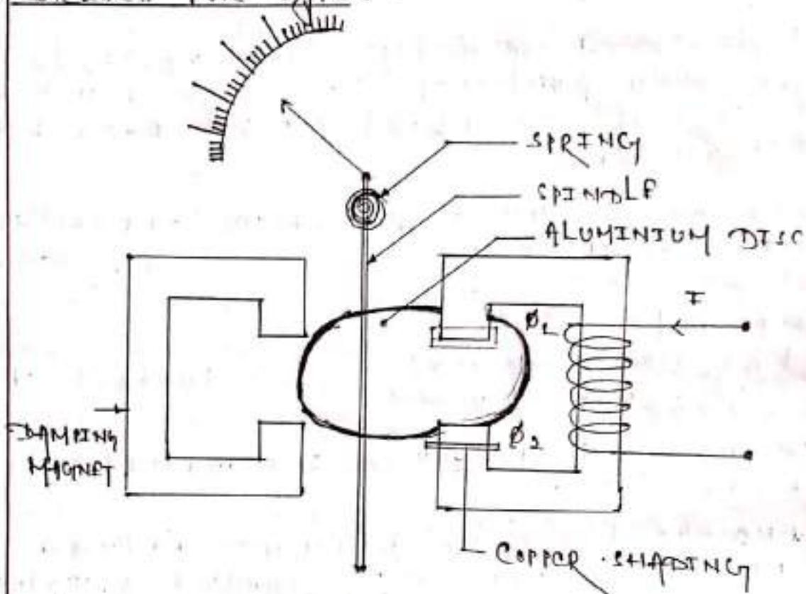
→ It consists of a metal disc which is placed in between the poles of an electro-magnet.
