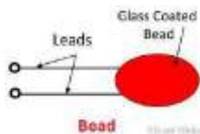
The bead form of the thermistor is smallest in shape.
