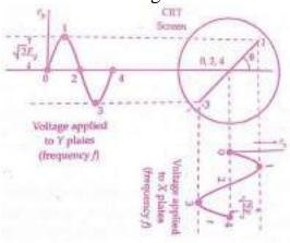
Figure: Lissajous figure for 0° phase shift
