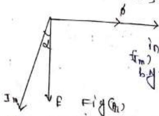
→ If the moving coil is assumed to be more inductive then current ( $I_m$ ) lags the voltage (E) by an angle  $\alpha$ .
