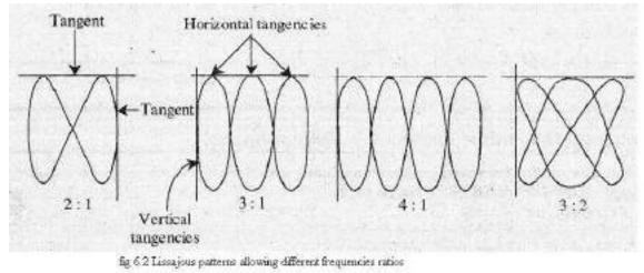
The ratio of frequency can be calculated by drawing tangent at top/bottom and left/right sides.
