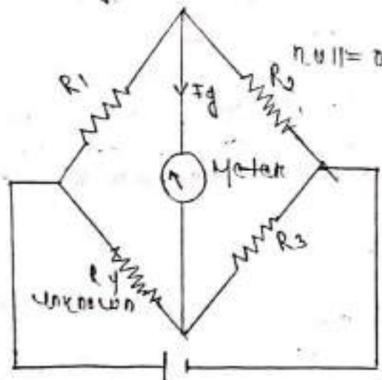
→ The current  $I_g$  is proportional to the unknown resistance  $R_4$ , when the bridge is unbalanced.
