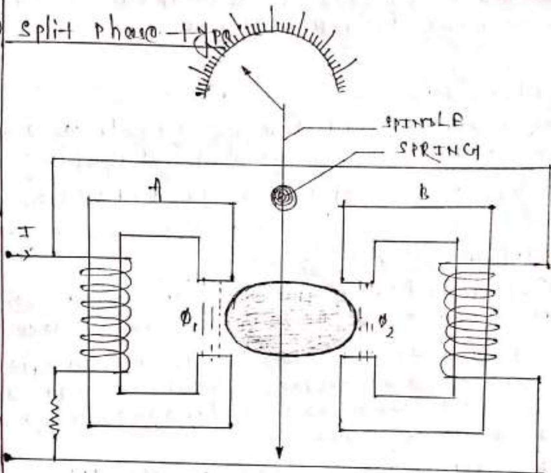
→ In this type of induction type instrument two electro-magnets are present to generate two fluxes  $\phi_1$  &  $\phi_2$ .
