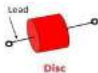
The disc shape is made by pressing material under high pressure with diameter range from 2.5 mm to 25mm
