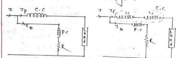
Fig! Electrodynamono ter - type watt moter.
