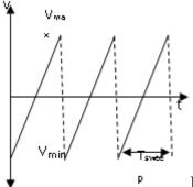
Figure: Sawtooth Waveform
