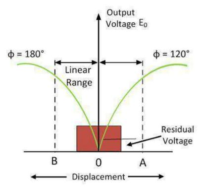
Figure: LVDT Characteristics
