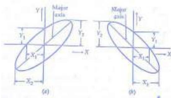
Referring to figure, the sine of the phase angle between the voltages is given by:
