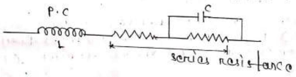
(ii) Error due to pressure coil capacitance:-
