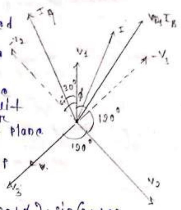
since the angular deflection of the pointer from the plane of reference is equal to the phase angle of the circuit, so the pointer movement can be calibrated in terms of power factor ( $\cos\phi$ ).
