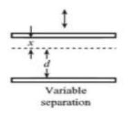
Since parameter 'd' changes, the capacitance 'C' also changes, as 'C' is inversely proportional to 'd'.
