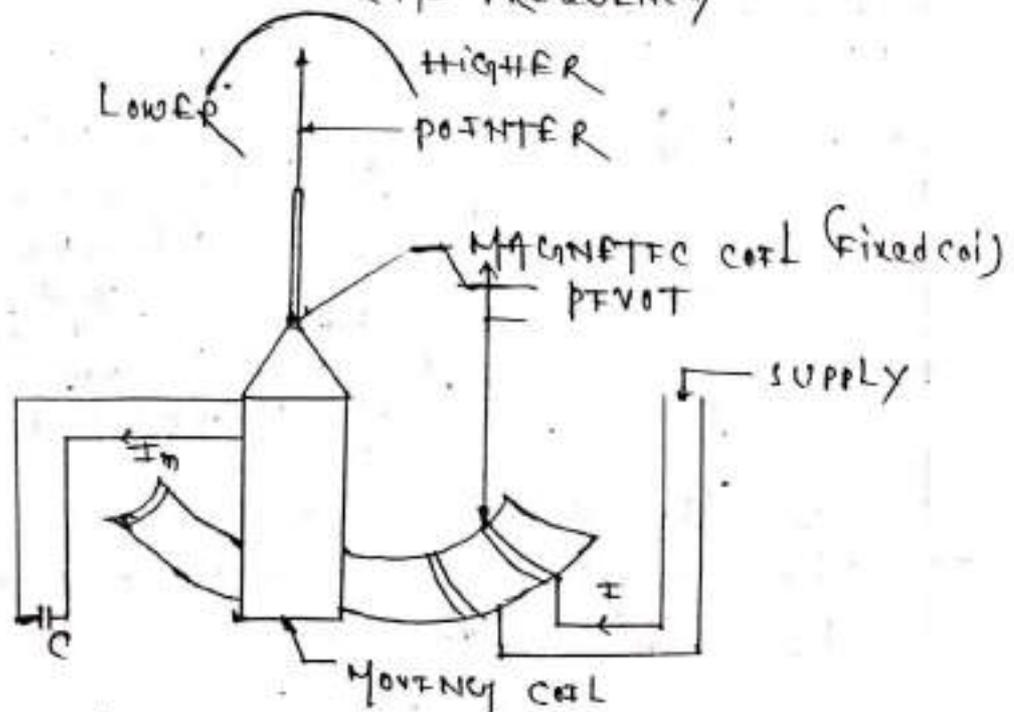
Fig: Ferrodynamic electrical resonance frequency meter.
