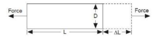
If  $\Delta L$  is the change in length of the wire by the application of force or stress then strain ( $\varepsilon$ ) is given by:
