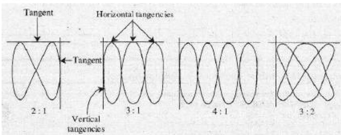
Fig 6.2 Lissajous patterns allowing different frequencies ratios
