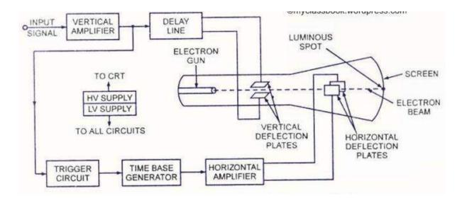
Figure: Block diagram of CRO
