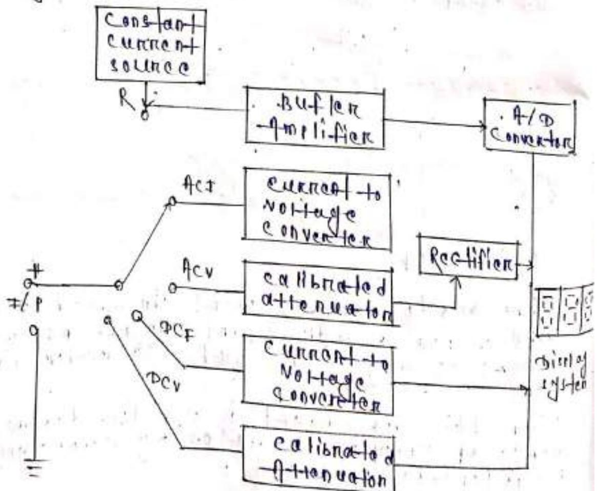
→ Digital multimeter is the instrument which is used to measure multiple quantity like :- voltage, current, resistance etc & display the measure quantity in terms of digits.
