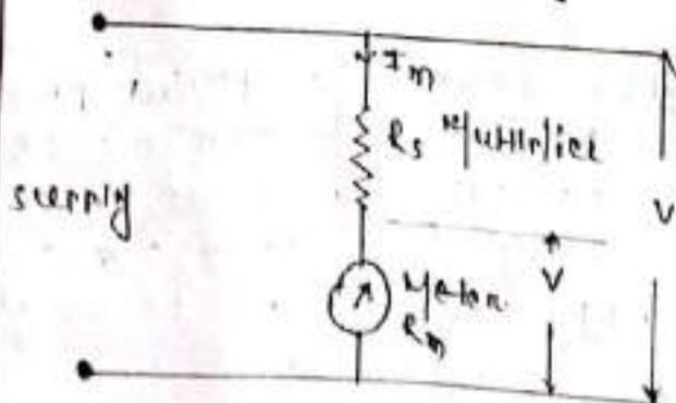
In the above diagram a series multiplier  $R_s$  is connected with the meter to extend the voltage range.
