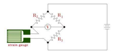
• In this circuit, R1 and R3 arms are equal to each other, and R2 is the rheostat arm and its value equal to the strain gauge initial resistance.
