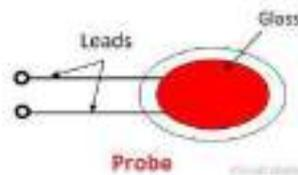
Bead type is enclosed inside the solid glass rod to form probes.
