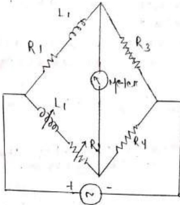
→ The Maxwell bridge measures inductance by comparing with a variable standard inductance.
