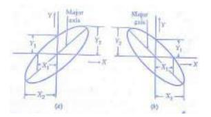
Referring to figure, the sine of the phase angle between the voltages is given by:
