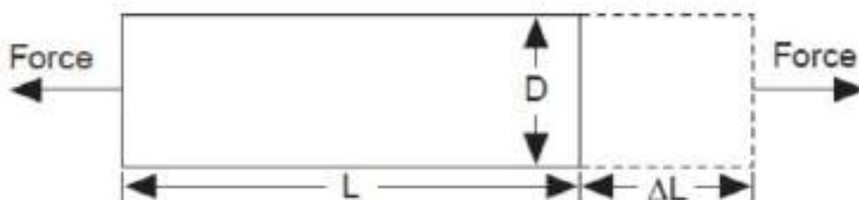
If  $\Delta L$  is the change in length of the wire by the application of force or stress then strain ( $\epsilon$ ) is given by:
