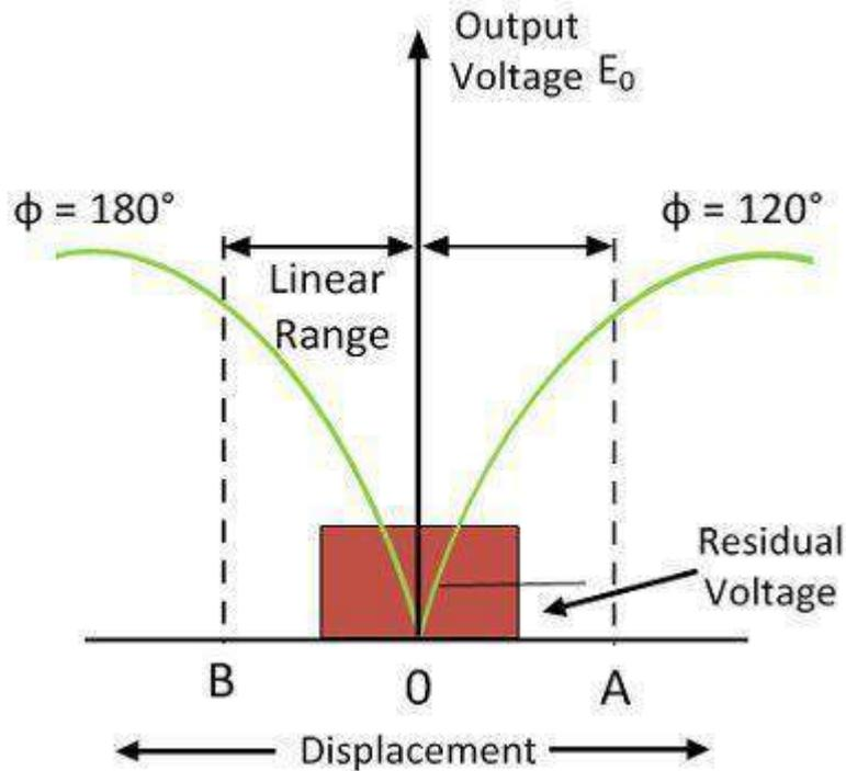
Figure: LVDT Characteristics
