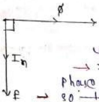
→ when the inductive reactance = the capacitive reactance then the circuit is under the resonance condition.
