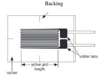
Figure: Wire type bonded strain gauge
