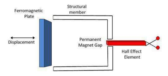
Measurement of Displacement Using Hall Efect Transducer
