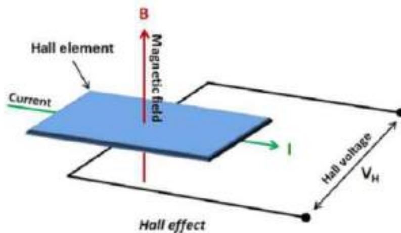
The output voltage of Hall Effect sensor  $V_H = K \frac{B \times I}{t}$
