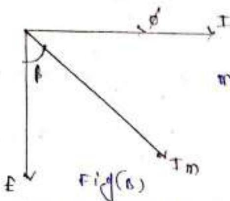
→ If the moving coil circuit is assumed to be more capacitive than the current ( $I_m$ ) leads the current ( $I$ ) by an angle  $\beta$ .
