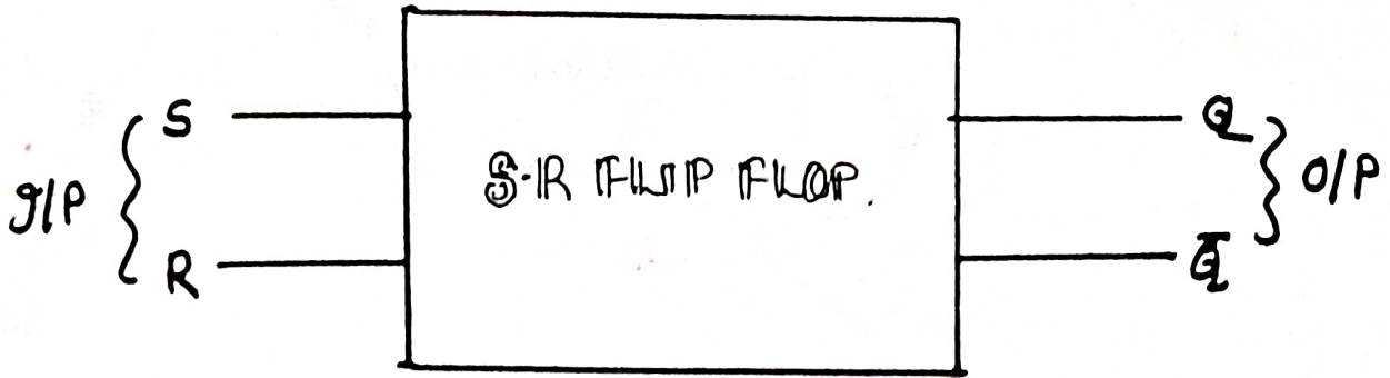
(BLOCK DIAGRAM OF S-R FLIP-FLOP).
