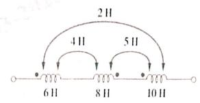
Find the total inductance of the three series connected coupled circuit.
