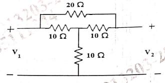
202001 Find  $l_1$ ,  $l_2$  and  $l_3$  by using Mesh analysis.
