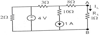
Determine the current through the load resistance 1 ohm using Norton's theorem.
