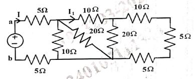
Find the Z-parameters of the circuit as shown in the figure. 3
