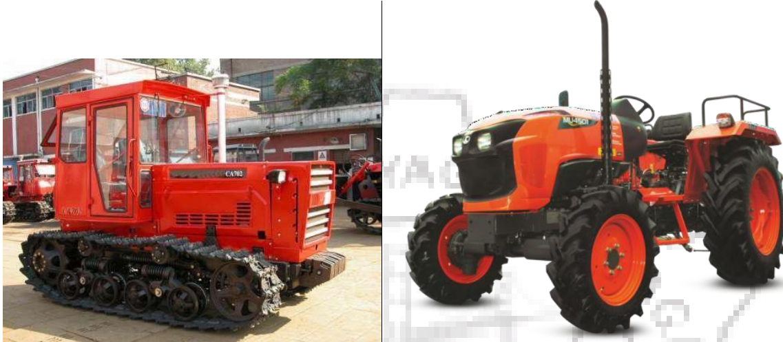
Fig. Crawler type tractor and Wheel type tractor
