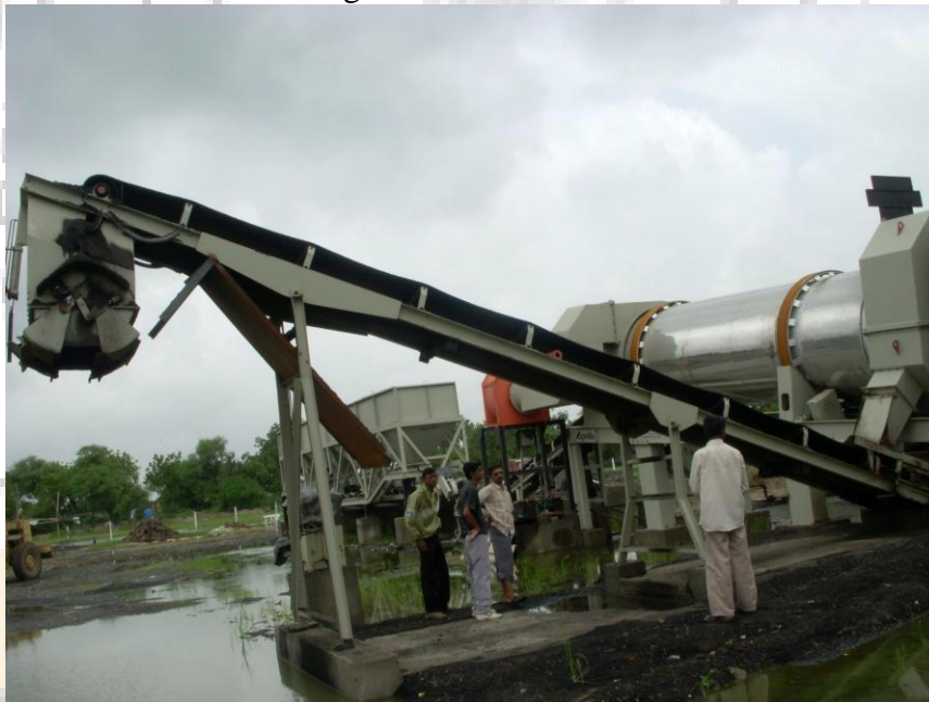
Fig. Load Out Conveyor
