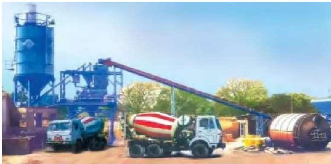
Modern ready mixed concrete plant.
