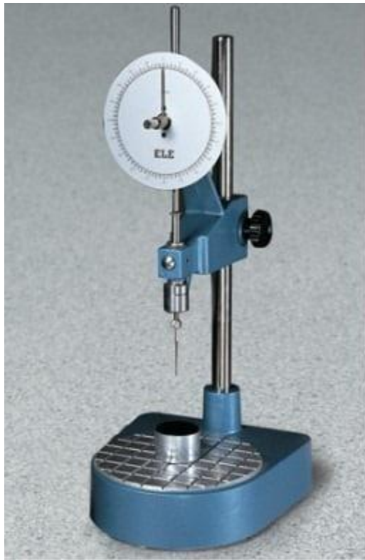
Fig:- Penetration apparatus and concept of penetration test.
