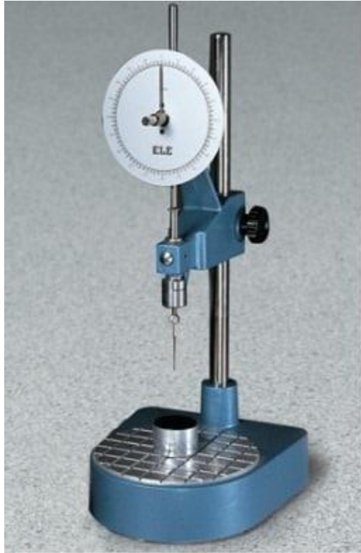
Fig:- Penetration apparatus and concept of penetration test.
